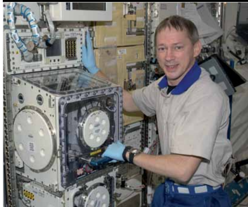
Frank De Winne works with the Space Linear Acceleration Mass Measurement Device (SLAMMD) in Europe's Columbus laboratory. SLAMMD is used to determine the body mass of crewmembers as part of ongoing medical investigations.
