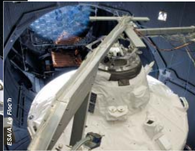
Jules Verne ATV undergoing tests in the Large Space Simulator at ESTEC in the Netherlands.
