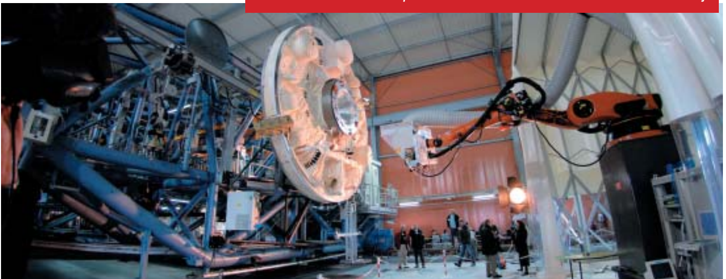
A 120 tonne mobile platform (left), mounted with a set of passive rendezvous targets (retroreflectors) identical to the ones installed on the ISS, facing the sensors mounted on an articulated industrial robotic arm (right). The relative motion achieved between the two is identical to that expected during rendezvous between the first Automated Transfer Vehicle Jules Verne and the Space Station. ESA/S. Corvaja
