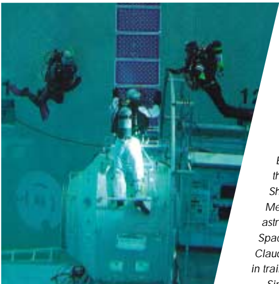
A special deep water pool – known as a neutral buoyancy facility – is used at EAC to train astronauts for working in space outside the Space Station.
