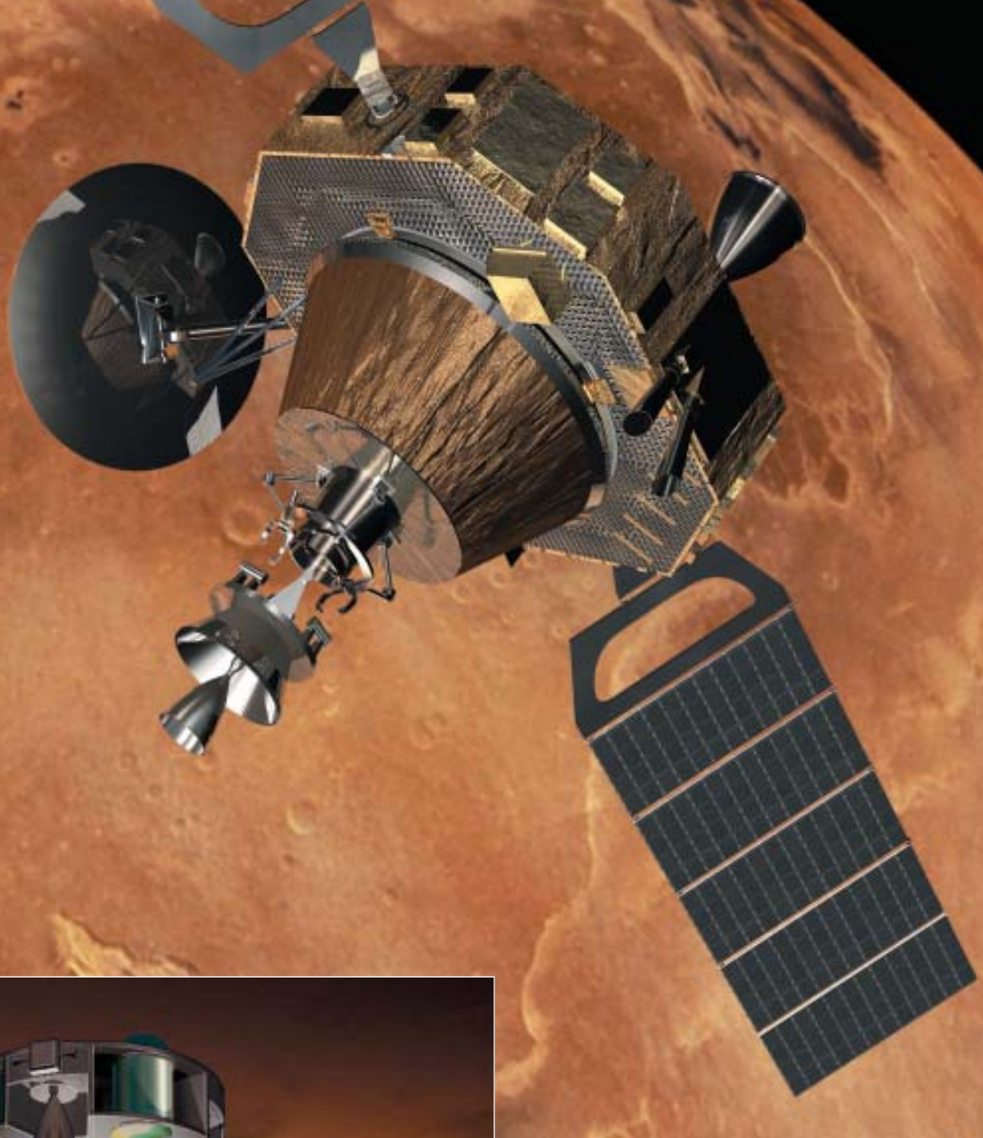
Artist's impression of Mars Sample Return Orbiter and (inset) an ascent module lifts off from the surface. ESA
