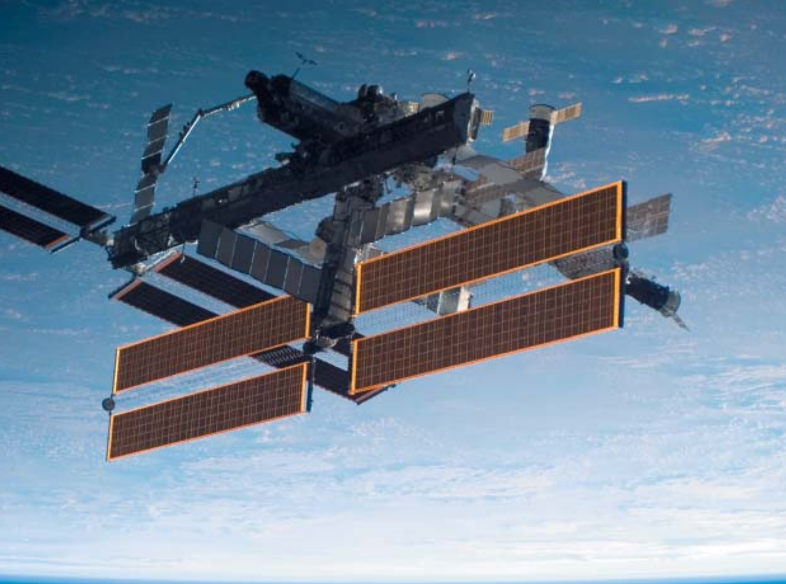
The ISS from Atlantis taken shortly after undocking, showing the ISS' new pair of solar wings attached to a new section of truss. NASA
