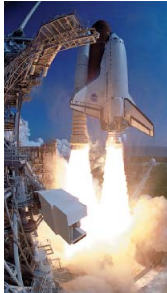
A fish-eye camera view curves the fixed service structure toward Space Shuttle Atlantis as it hurtles past, propelled by columns of fire from the solid rocket boosters. Below, the smoke and steam billows across Launch Pad 39B. At the lower left is the White Room that, when extended against Atlantis, gave the mission crew access to the orbiter. NASA
