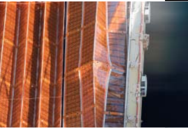
An image of a kink that occurred in the port-side P6 solar array during the first attempt to retract it on 13 December. The crew later extended the array and managed to clear it.
